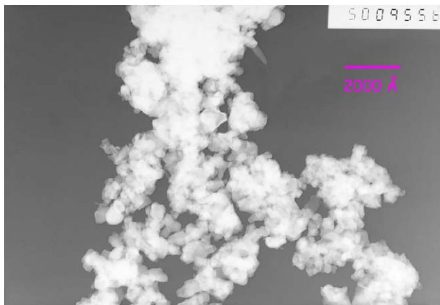
Fig. 2. Transmission electron microscope image of the gadolinium gallium oxide powder heat treated at 800 °C for 30 h. The viewgraph shows a microstructure with features in the 500–700 Å range size.
